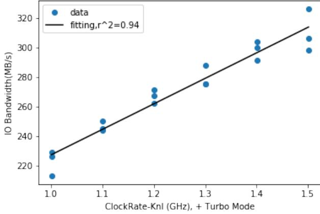
Fig. 8. KNL IO Bandwidth vs. CPU Frequencies (with Turbo Mode), Page Cache On
