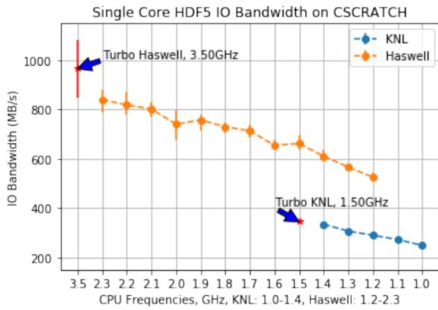
Fig. 4. Buffered IO Performance with Varying CPU Frequencies, HDF5
