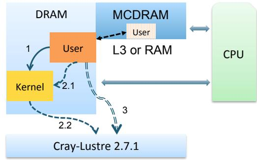
Fig. 2. IO Path on KNL, 1/2/3 is buffered/synchronous/direct IO; User data is located in either MCDRAM or DRAM and depends on MCDRAM mode and NUMA configuration
