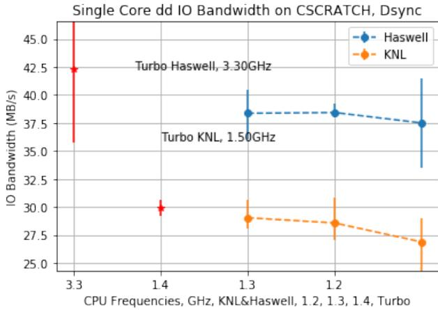
Fig. 9. IO Bandwidth vs. CPU Frequencies (with Turbo Mode), Synchronous IO
