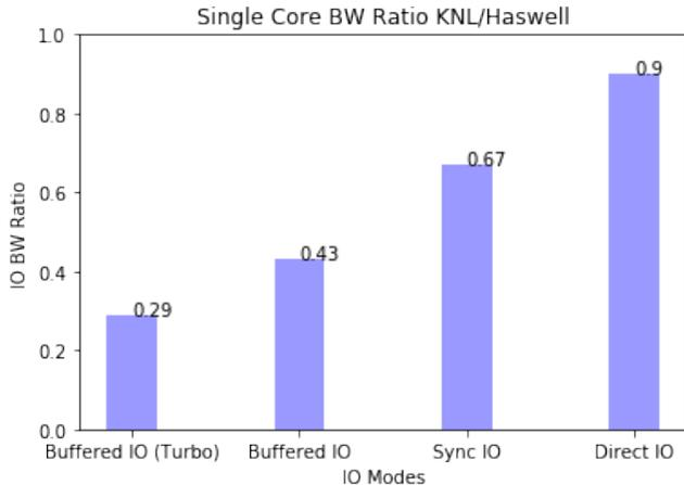
Fig. 12. Performance Ratio between KNL and Haswell with different IO mode
