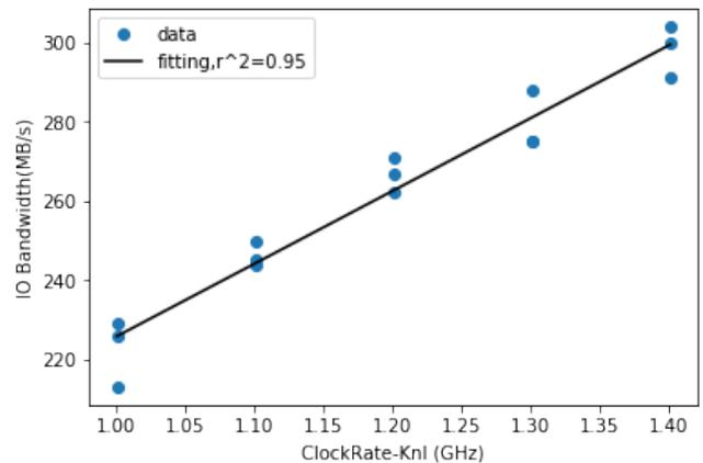
Fig. 7. KNL IO Bandwidth vs. CPU Frequencies, Page Cache On
