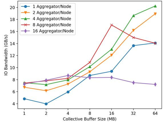
Fig. 19. Haswell IO Bandwidth with different collective buffer size and aggregators per node.
