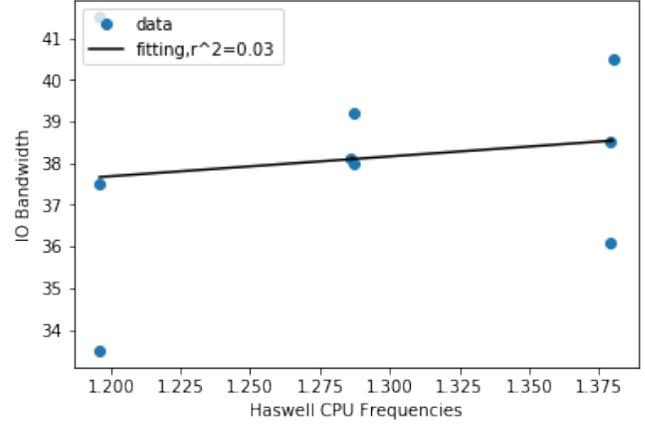
Fig. 10. Haswell IO Bandwidth vs. CPU Frequencies, Synchronous IO
