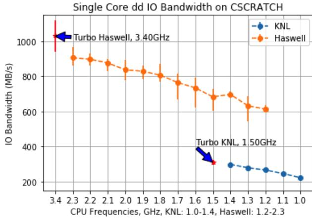
Fig. 3. Buffered IO Performance with Varying CPU Frequencies, dd
