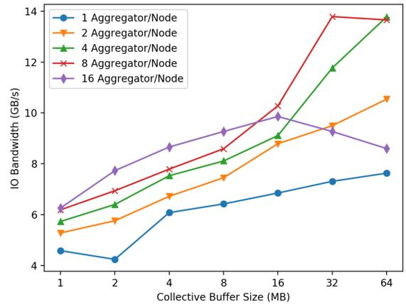
Fig. 20. KNL IO Bandwidth with different collective buffer size and aggregators per node.
