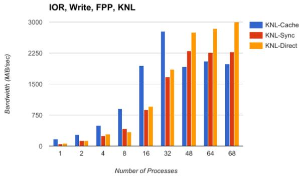
Fig. 16. IOR File Per Process Write on KNL, Weak Scaling on Single Node
