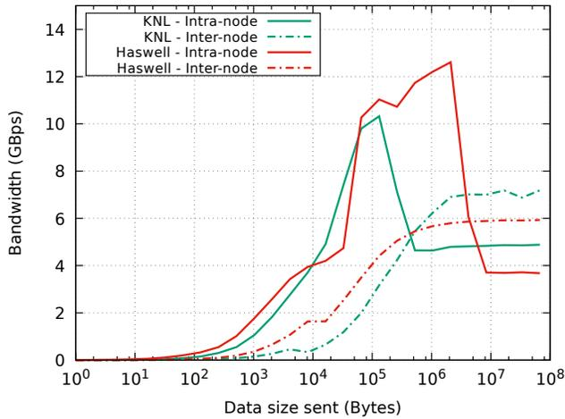
Fig. 18. Bandwidth comparison for KNL-based and Haswell-based nodes for a ping-pong benchmark with intra-node and inter-node communication
