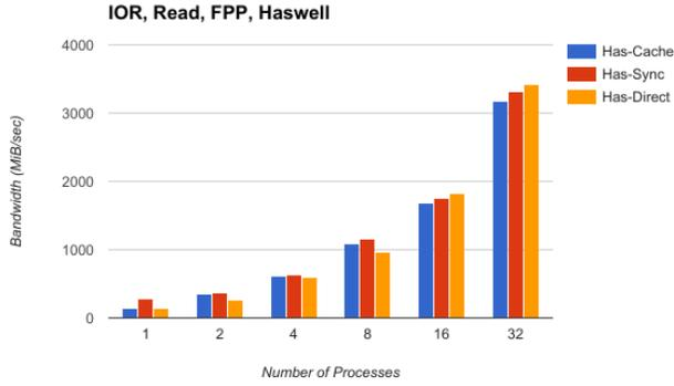
Fig. 15. IOR File Per Process Read on Haswell, Weak Scaling on Single Node
