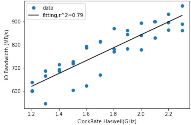
Fig. 5. Haswell IO Bandwidth vs. CPU Frequencies, Page Cache On
