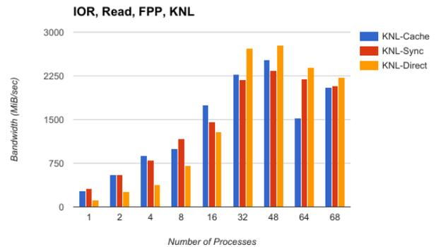
Fig. 14. IOR File Per Process Read on KNL, Weak Scaling on Single Node
