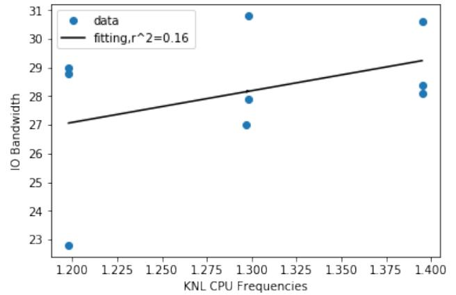
Fig. 11. KNL IO Bandwidth vs. CPU Frequencies, Synchronous IO
