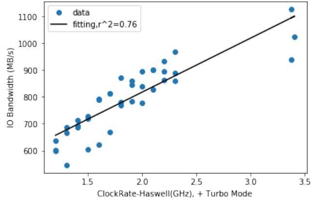
Fig. 6. Haswell IO Bandwidth vs. CPU Frequencies (with Turbo Mode), Page Cache On
