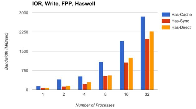
Fig. 17. IOR File Per Process Write on Haswell, Weak Scaling on Single Node
