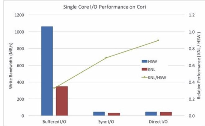
Fig. 13. Performance Ratio between KNL and Haswell with different IO mode, (a different view)
